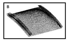
Fig. 3 — Distortion shape due to bending and buckling under mechanical load. A — Bending distortion (30.5-cm panel); B — buckling distortion (101.6-cm panel).
