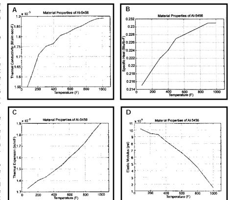
Fig. 13 — Temperature-dependent thermal properties of AI-5456-H116 used in the FEA studies (Refs. 16–19). A — Thermal conductivity; B — specific heat; C — thermal expansion coefficient; D — elastic modulus.
