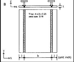
Fig. 1 — Stiffened panel under mechanical and thermal loads for buckling analysis. A — Mechanical model; B — thermal model.
