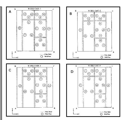
Fig. 14 — Welding sequences for angular distortion analysis of aluminum panel structure. A — Welding sequence No. 1; B — welding sequence No. 2; C — welding sequence No. 3; D — welding sequence No. 4.
