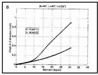
Fig. 2 — Load-displacement curves under mechanical load (width = 30.5 and 101.6 cm, length = 101.6 cm, thickness = 6.4 mm). A — Bending distortion (30.5 cm panel); B — buckling distortion (101.6-cm panel).
