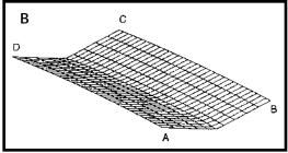
Fig. 10 — Final deformation shape on the back side of the T-flange. A — Measurement grid and measured deformation; B — calculated deformation using the inherent shrinkage method.
