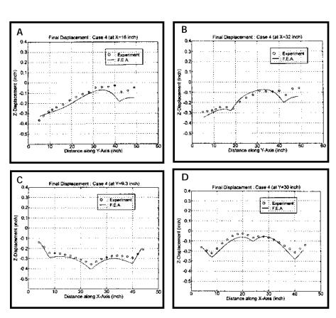
Fig. 17 — Comparisons between predicted and measured distortions along four cross sections in the aluminum panel, welding sequence No. 4. A — At x = 40.6 cm; B — at x = 81.3 cm; C — at y = 23.6 cm; D — at y = 76.2 cm.
