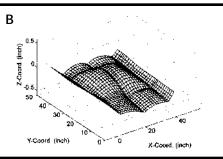
Fig. 15 — Distortion shape resulting from welding sequences No. 2 and No. 4. A— Welding sequence No. 2; B — welding sequence No. 4.
