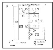
Fig. 20 — Joint rigidity indices at the unwelded joints. A — After 6th weld pass; B — after 12th weld pass.
