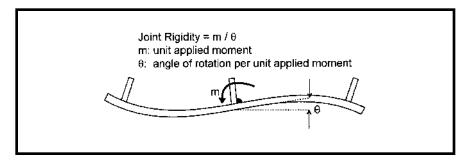
Fig. 18 — Definition of joint rigidity.
