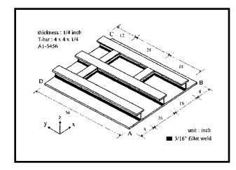
Fig. 12 — Aluminum panel for study on welding sequence effect on angular distortion.
