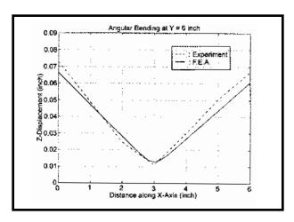
Fig. 11 — Comparison of angular distortion on the back side of the T-flange determined by the inherent shrinkage method and experimental measurement.
