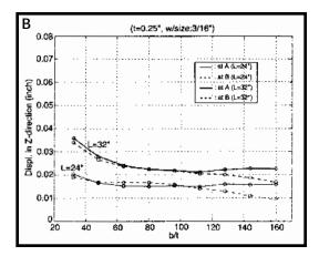
Fig. 4 — Displacement curves under thermal load (width = 101.6 cm, length = 101.6 cm). A — Thickness: 3.2 mm; B — thickness: 6.4 mm.
