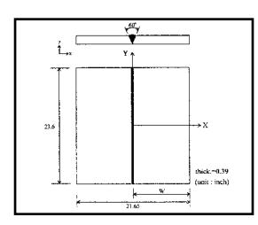
Fig. 6 — Butt joint groove-welded rectangular aluminum plate for residual stress characterization (Ref. 6).
