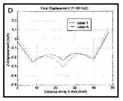
Fig. 21 — Comparison of distortions resulting from welding sequence No. 1 and the optimum welding sequence A. A — At x = 40.6 cm; B — at x = 81.3 cm; C — at y = 23.6 cm; D — at y = 76.2 cm.
