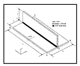
Fig. 9 — Aluminum T-joint specimen for angular distortion characterization.
