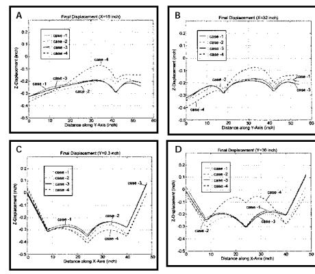
Fig. 16 — Distortion displacements at four cross sections of the panel from four welding sequences. A - At x = 40.6 cm; B - at x = 81.3 cm; C - at y = 23.6 cm; D - at y = 76.2 cm.
