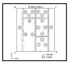
Fig. 19 — Optimum welding sequence (sequence A) determined by JRM.
