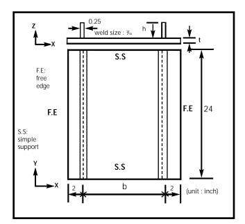
Fig. 5 — Stiffened aluminum panel for residual stress characterization.
