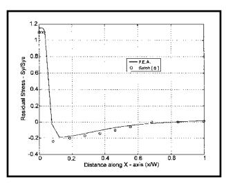
Fig. 7 — Comparison of longitudinal residual stresses determined by the inherent shrinkage method and experimental measurement.
